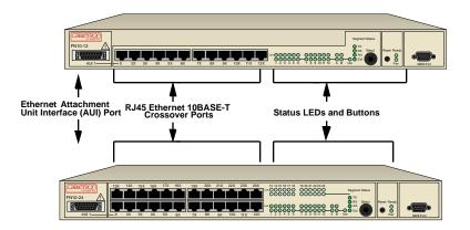
Figure 2-1 FN10 12- and 24-Port Front Panels
